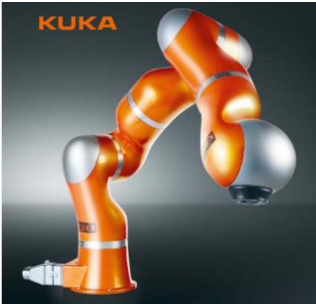
Figura 5.1: Brazo robótico KUKA Lightweight 4+.
